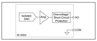
Figure 4. Output Circuitry for One Channel of the NI 9264
